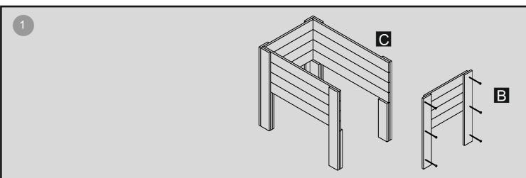
Place and fix the end sections against the sides using six screws as shown. Make sure that you pre-drill first and that the screws are fully located in to the material.
