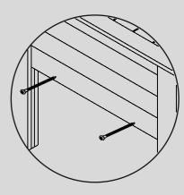
Place the base in to the planter so that it rests on the legs. Fix the base to in place screwing through each side using four screws spaced evenly. Make sure that you pre-drill first and that the screws are fully located in to the material.
