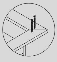
Place each of the cills on to the planter and fix at the corners using two screws for each. Further secure these using a single screw midway down each cill, screwing in to the board.
