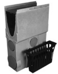
ACO M200DS universal sump with plastic silt bucket
