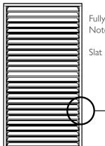
Fully framed with a steel mechanism. Note: slats do not close fully.
