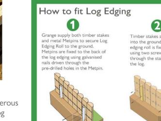
Timber stakes are driven into the ground and the edging roll is fixed to them using two screws to go through the stake into
