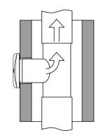
To maximise airflow rigid ducting should be used. Where flexible ducting is used the diameter must be maintained and it is good ventilation practice that the ducting is extended to 90% of its possible length in order to maintain the best possible airflow. Ensure that flexible duct connections are not over tightened to the fan outlet spigot. The fan and ducting when installed should perform in accordance with the requirements of UK Building Regulations Part F Volume 1: Dwellings.
