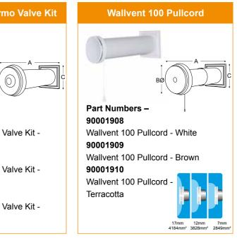
• The Wallvent 100 Pullcord offers manual volume flow adjustment using an integrated free-hanging pull cord with a three-level locking mechanism. The supply air flows in through the disc valve and is optimally distributed into the habitable room.
