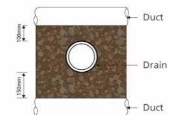
Minimum clearance between duct and drain
