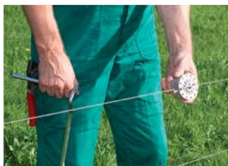
Insert the rotating wire tensioner in the wire, attach the wire tensioner handle
