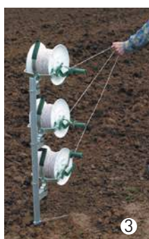
3 Take the polywires from the reels and unwind
