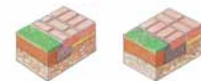
Edging with a double block string course Edging with a block soldier course
