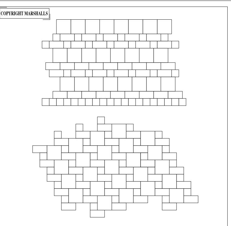
Suggested layout using: 600x600mm x 24 No. 600x297mm x 35 No. 297x297mm x 34 No.
