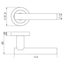
Lever on concealed fix 2 part screw on round rose. A plain straight round bar lever which is easy to grasp and operate comfortably. Its minimalistic lines will look good in any environment. Comes with a 10 year mechanical guarantee and is Fire door rated.
