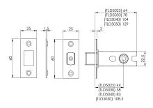
Tubular Dead Bolt. with either 5mm or 8mm follower option. Commonly used as a bathroom deadbolt using a separate turn and release. Certified to BS EN 12209.
