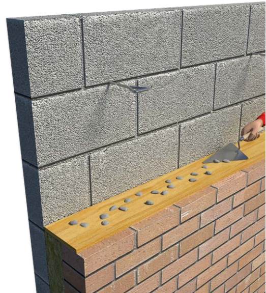
Figure 2 Use of a cavity board when clearing off mortar
