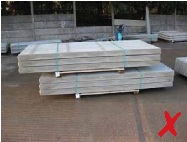
Products MUST be stacked on top of each other, keeping the load bearers in line.
