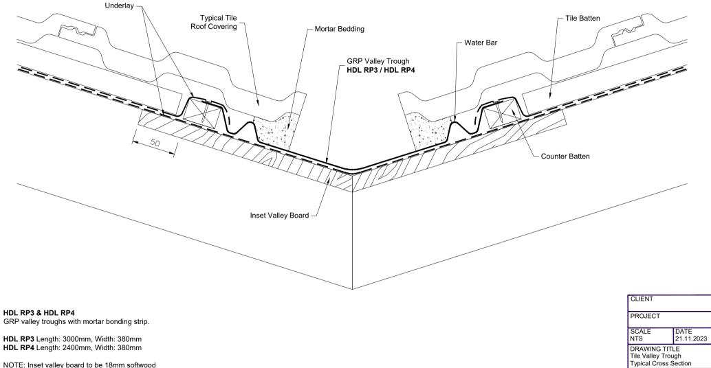
HDL RP3 Length: 3000mm, Width: 380mm HDL RP4 Length: 2400mm, Width: 380mm
