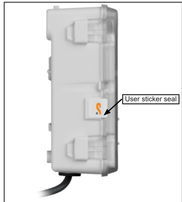
Figure 7-17: User sticker seal on assembled integrator unit
