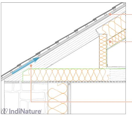
Ensure there is a 50mm ventilation gap between the sarking board and IndiTherm between the roof joists.
