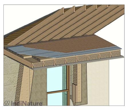
Cold roof loft insulation is one of the most effective ways to reduce heat loss through the building fabric. Batting should be at least 300mm deep to achieve maximum performance. Batting should be layered perpendicularly to perform most effectively. A vapour permeable membrane can also be laid on top to prevent air circulation through the batting which can draw heat through the insulation and reduce it's efficacy.
