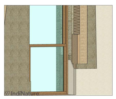
Window reveals are an especially tricky point to insulate as there is very limited space. Stripping back the original finish will provide extra space in which a rigid insulating board may be fitted. Tapered rigid insulation boards are provided by other manufacturers which are ideal for this situation.
