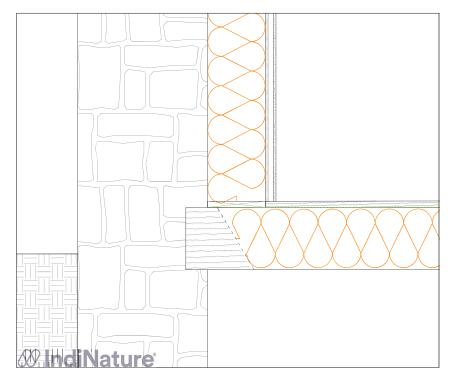
IndiTherm should be installed in between studwork which can be finished in a number of ways. Current advise is to install 140mm of IndiTherm to meet current Building Regulations.
