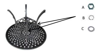
Attach the Table legs Support (③)to the four Legs (②)using flat washer, spring washer and nuts(A,B,C)
