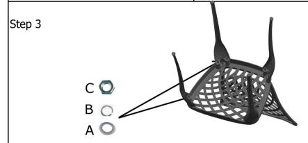
Attached the legs(③)onto the Chair Seat(②)using washers, Spring washers and Nuts(A,B,C). Tighten the nuts using the Wrench(⑥)
