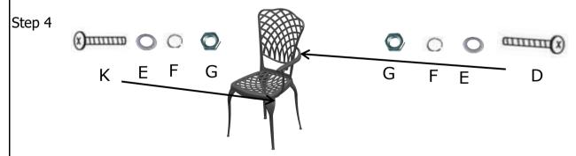
Attach the Right arm and Left arm (4&5) to the Chair Seat (2) using Stud(K) washers,spring washers and nuts(E,F,G),DO NOT over tighten. Then Connect the Backest(1) using Stud(D),Washers and Nuts (E,F,G).Tighten the Nuts using the wrench .Adjust all bolts and let all right directions.Tighten the bolts.
