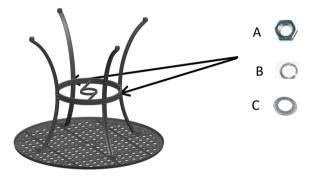
Attach the Table legs Support (③)to the four Legs (②)using flat washer,spring washer and nuts(A,B,C)
