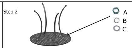
Turn over the table top.Attach the Stud M8(E) into the Nuts(inside table),Then,Attach table Legs(②) to the Studs on the Table Top (①) using Wahers and Nuts (A,B,C).DO NOT over tighten
