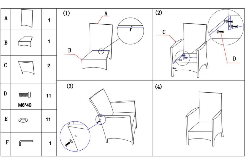
Important: Do not fully tighten all screws until assembly is complete.
