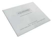
AQUAPANEL® Interior Cement Board is a solid, durable tile backing board for interior use in wet and humid areas. It is made of aggregated Portland cement with coated glass fibre mesh embedded in the back and front surfaces. The board ends are cut square and edges are reinforced for extra strength (EasyEdge®).
