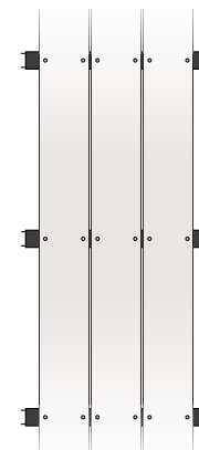
Fixed twice using Cedral colour matched screws
