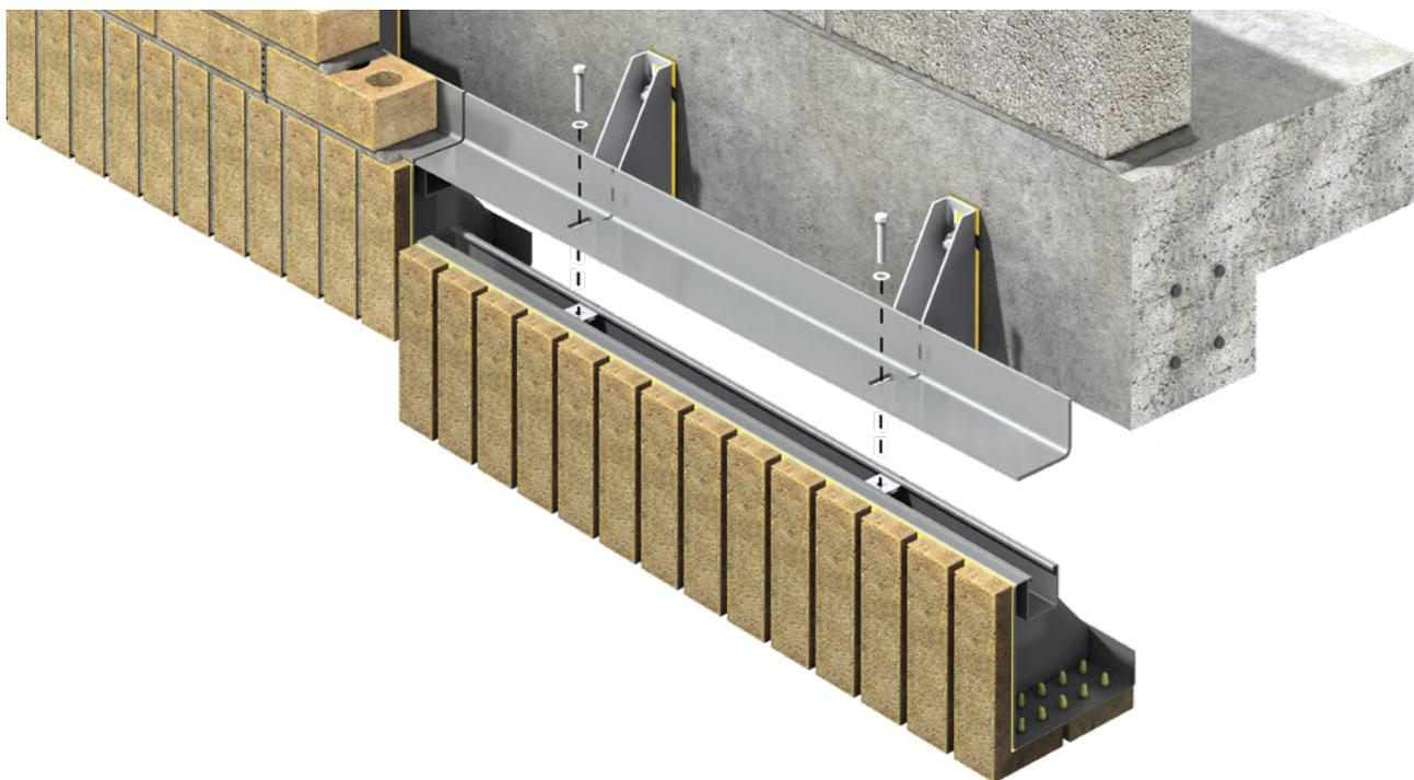
By combining our Keystone masonry support system with bespoke steel components we produce single and double sided soffit systems which are ideal for runs of any length.
