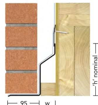
T/K-70 W = 68mm - for 70 to 85mm cavity widths
