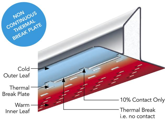
Standard Keystone Lintel with patented non continuous Thermal Break Plate
