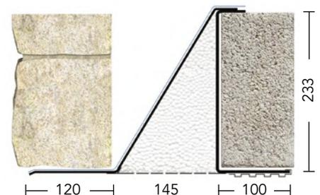
Cavity widths from 50mm-165mm
