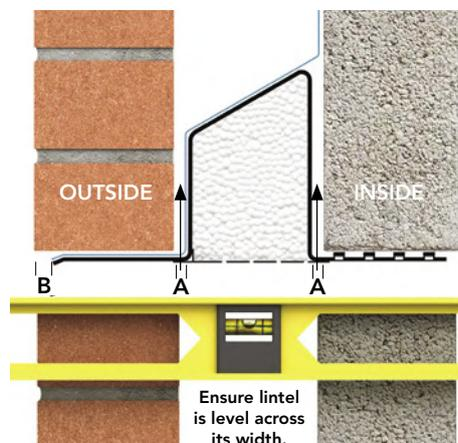
In accordance with BS EN 1996-2:2006 and NHBC requirements all external wall lintels **MUST** be installed with a flexible damp proof course with the exception of those adequately protected by an eaves overhang or similar form of protection.
