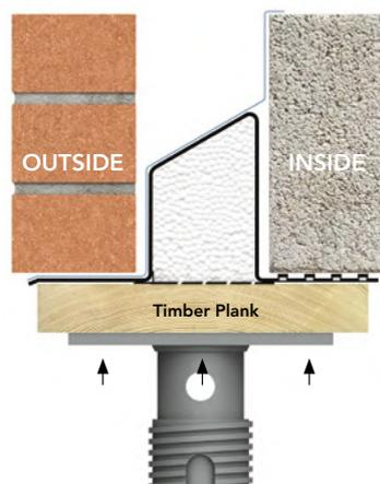
The practice of propping a lintel is sometimes used to facilitate speed of construction. It should only be introduced after initial masonry load has been applied to the lintel.
