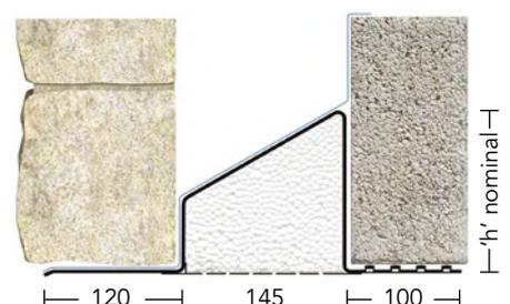
Cavity widths from 50mm-165mm
