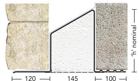
Cavity widths from 50mm-165mm
