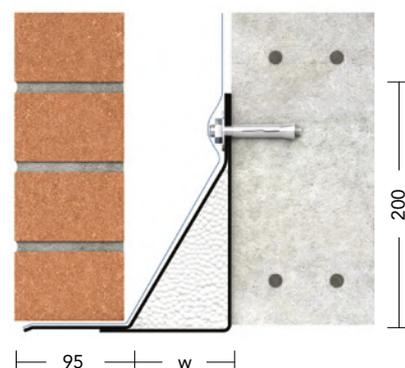
W = cavity width of 75mm or 100mm
