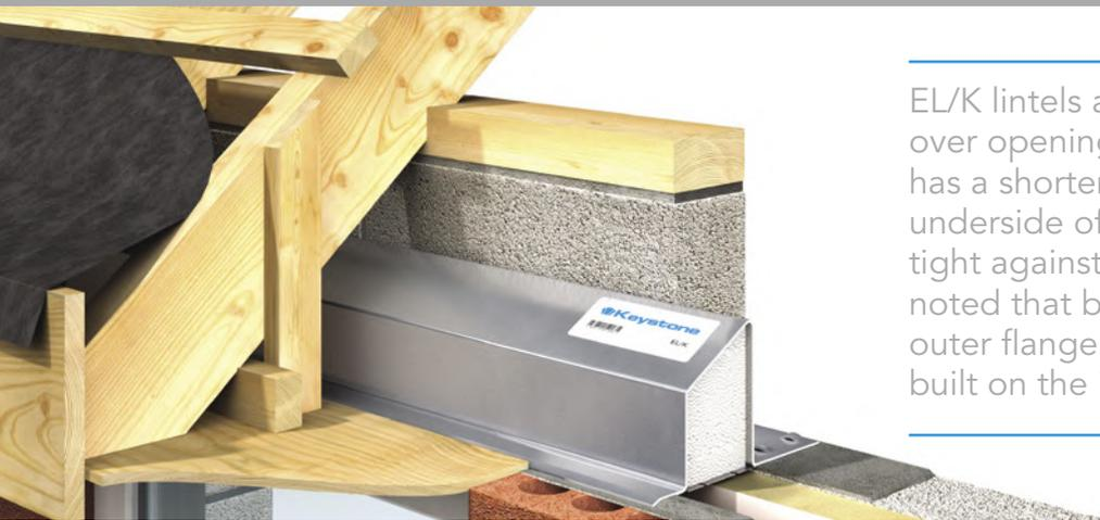
EL/K lintels are designed to provide support over openings at eaves level. The eaves lintel has a shortened outer flange to allow the underside of the soffit board to be positioned tight against the window frame. It must be noted that brickwork cannot be built onto the outer flange of an eaves lintel. Masonry is built on the inner leaf only.
