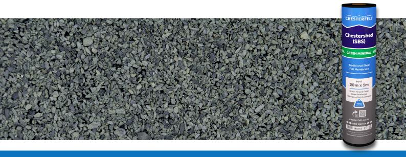
Chestershed Mineral SBS is a waterproof protection layer for use on portable type buildings with pitched roofs, such as sheds, stables, kennels and non-inhabited buildings. It features a glass fibre base which is saturated and coated in SBS modified bitumen and finished with light sand on the lower surface and green mineral granules on the upper surface.
