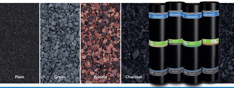
Deflector is a multi-layered bituminised waterproof system designed for use on various types of flat roofing projects including new build and refurbishments, cold roofs and warm roofs using vapour control layers with insulation. This range of membranes feature a polyester core which is saturated and coated in SBS modified bitumen and the upper surface is finished with a choice of either light sand or slate mineral.
