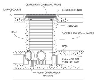
Clark-Drain inspection chambers CD 453 and risers CD 455 are designed and manufactured to BS EN 13598-1:2010. Chambers may be filled to ground level (1.2 metres max) in isolation or as part of a pipeline or complete drainage installation.
