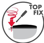
Top fixing is required when there is a limited/no access to the underside of the hinge mounting holes (blind hole pans).
