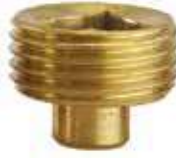
Air Vents 13mm ½" WITHOUT KEY • Brass with BSP male parallel thread • 10bar max
