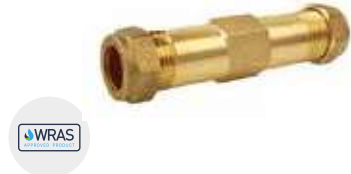
Repair Coupler BRASS COMPRESSION REPAIR COUPLER • Suitable for use with hot/cold water and central heating systems • Manufactured to BSEN1254-2 • WRAS Approved
