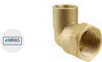
FI Elbow SOLDER RING FEMALE IRON ELBOW • Suitable for use with hot/cold water and central heating systems • Manufactured to BSEN1254-1
