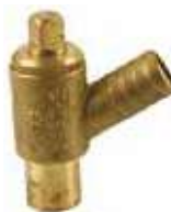
Type A Capillary Long Draincock TYPE A CAPILLARY LONG DRAINCOCK 15mm TAIL SHANK • Sturdy brass construction • Supplied with seal inside body, this keeps the product watertight when not in use • No need for a specific key to tighten • Water flow can be easily adjusted by use of a spanner
