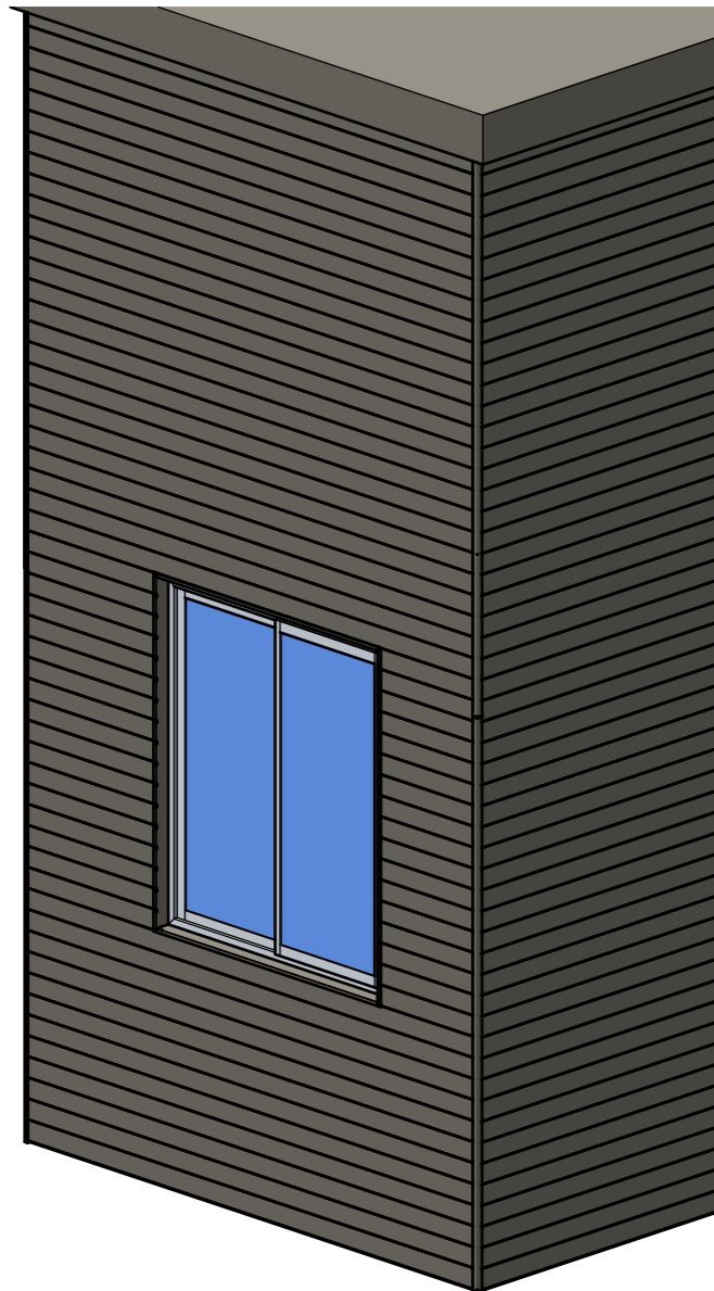
Iso: Cladding Corner Detail - showing internal corner and interface of vertical slatted cladding with a render or brick wall finish
