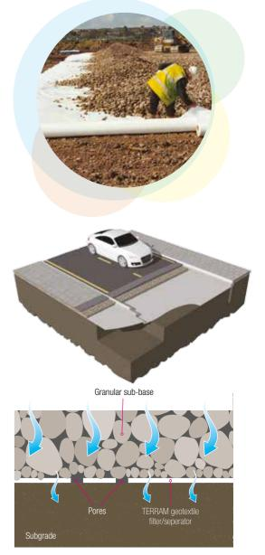
A natural filter is established adjacent to the geotextile's pores.
