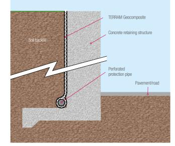
Retaining Structures. To maintain the stability of a retaining structure it is important to provide an efficient drainage system at the rear of a retaining structure to prevent the build up of pore pressure.
