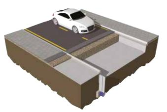
Vertical edge drains running parallel to a roadway are necessary to intercept the lateral flow of groundwater. A geocomposite fin drain saves on excavation and is quicker to install than a stone alternative
