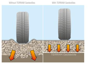
Intermixing of the sub-base and subgrade prevents the full load- bearing capacity of the stone layer being mobilised and leads to failure. A suitable geotextile acts as a filter separator throughout the highway's life and acts to preserve the stone layer's integrity.
