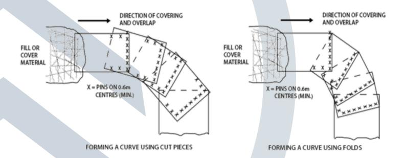
Overlaps around curves should be formed from short cut sections or folded sections of fabric. These should be overlapped and offset one edge versus the other such as to turn the fabric path around the corner. Sections should be anchored or pinned to the ground. See diagram above.
