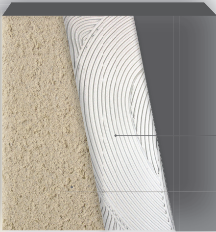
1 layer of PRB RÉNOMUR TOP left with a serrated finish Single-coat render finish
