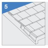
Slide the next verge unit into the upper edge of the first unit. Press firmly to the tile fitting it under the head laps to ensure the unit is firmly held in place. Screw the unit through the top grid into the batten.
