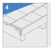
Slide the first verge unit over the tile at the eaves and into the starter kit fitting it under the head laps to ensure the unit is firmly held in place. Fix the unit through the top grid into the batten with a 40 x 3.35mm
