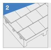
Set tiles flush with the battens. For refurbishment projects remove existing mortar bedding and install new tiling batten to the underside of the existing tiling batten.
