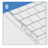
Continue the process along the barge board to the ridge. Now insert the ridge cap once the final verge is completed so that the last nail plate is covered.
