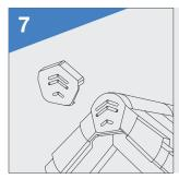
The half-round ridge end cap (code ULTI2ECR) or universal angle ridge end cap (code ULTI2ECA) should be fitted interlocking with the verge units and then screw fixed into the barge board or masonry, unless a Tile Manufacturers Block End Ridge is being utilised.
