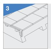
Starting at the bottom edge of the roof, insert the starter piece (remove tab to suit as shown below) into the front end of the verge unit and mark out the starter position on the fascia and barge board. Remove the unit and mechanically fix the starter piece into position through the grid with a 40 x 3.35mm screw.
