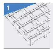
Install the tiling battens with a **40mm** overhang over the brick or barge board. For refurbishment projects install a new tiling batten to the underside of the existing tiling batten.
