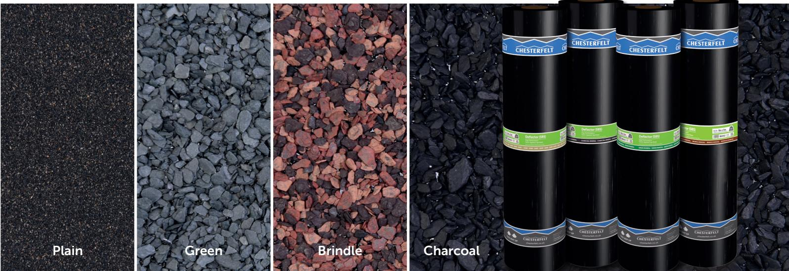
Deflector is a multi-layered bituminised waterproof system designed for use on various types of flat roofing projects including new build and refurbishments, cold roofs and warm roofs using vapour control layers with insulation. This range of membranes feature a polyester core which is saturated and coated in SBS modified bitumen and the upper surface is finished with a choice of either light sand or slate mineral.
