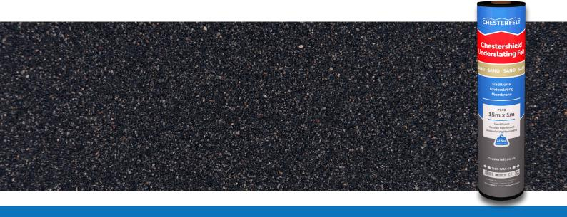
Chestershield Underslating Felt is a traditionally manufactured, hessian-backed felt for use under tiles or slates. Its fibre base is fully impregnated with a penetration grade bitumen in a saturation bath prior to being jointed with a jute hessian in the coating section.
