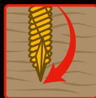
Rapid Drive Twist Cut Enhances Drive Performance
