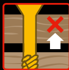
Partially Threaded Stops The Timber Jacking
