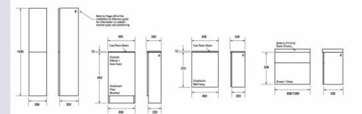
Please Note: Letters 'A' 'B' & 'C' indicated in units are for positioning of wall hanging brackets. Please use diagrams on page 9 of your Installation & After Care Guide for dimensions showing fixing positions.
