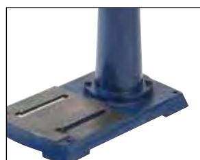
Sturdy base and column connection. (Column diameter 70mm)
