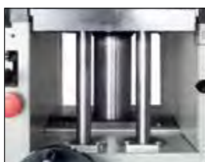
Thicknessing bed mounted on centre ram and additional supports for even and stable thicknessing
