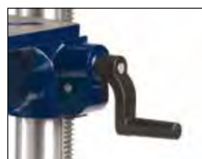
Workbench height adjustment, thanks to a rack.
