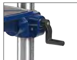
Workbench height adjustment due to a rack
