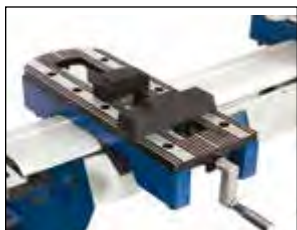
Two part clamping system to hold workpieces
