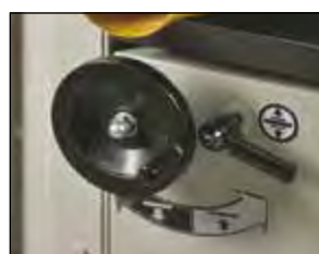
Rise and fall handle with height lock
