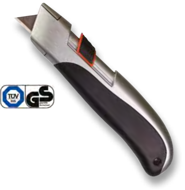
Even if slider is still at extending position, blade retracts automatically when it loses contact with material being cut.
