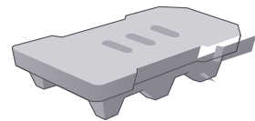
T2: 700 x 347mm (Chamfered corners 70 mm @ 45° one end)
