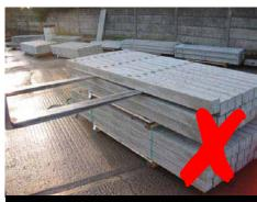
Products must not be taken out of packs using the forklift, they will damage the unit
