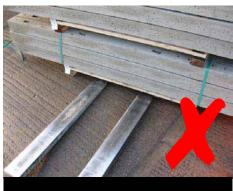
The forks must not be close together when picking up packs
