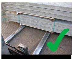
The forks must be widened to be as close to the load bearer as possible
