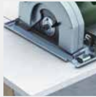
Figure 3: Sawing with circular handsaw
