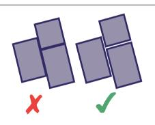
Never butt joint paving when laying you should always use an appropriate joint for your chosen product. Global Stone products should be laid with a minimum 8-10mm joint.
