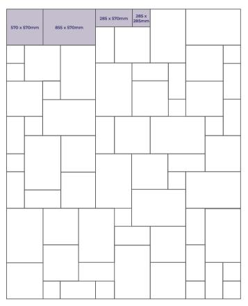
All dimensions shown are nominal, pattern includes 10mm joints approximately. Always mix slabs (whilst laying) when using multiple packs.
