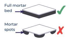
Always lay paving on a full bed of mortar and never use the spot bed method – see our step by step laying guides for more advice on this.
