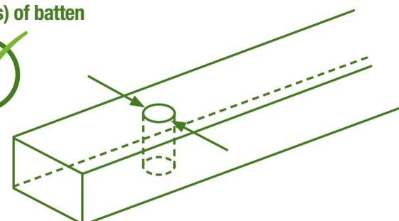
The rule on knots can be quite complicated, but essentially, any large knot which is bigger than half the width of the batten, appearing on both sides of the face (width), as illustrated above, would not be compliant to BS 5534.
