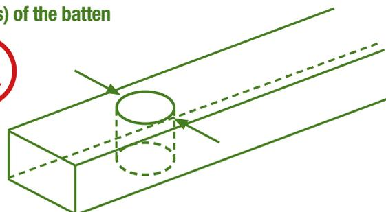
**Less than half size on both faces (widths) of batten**
