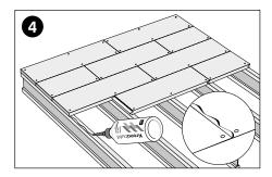
Repeat the application steps on subsequent rows of boards which should be laid in a staggered pattern. Short end joints, including perimeter edges, must fall on a secured joist or noggin. The boards must be fixed at the rate of three per board (i.e., one at each end and one in the middle). This nailing pattern gives a mechanical fixing every 1200 mm along each joist. Any excess adhesive should be left to dry then removed at the end of the build process. If in doubt consult NHBC guidelines.
