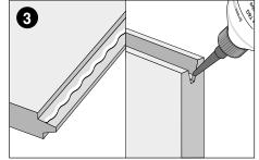
Apply Kronobuild® D4 Adhesive along the full length of both the tongue and groove profile as boards are fitted. The joints should be securely bonded when the boards are interlocked.
