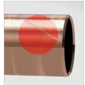
4. Check for scratches and scores
