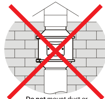
Do not mount duct or motor vertically
