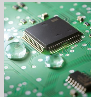
Conformal coated waterproof PCB board
