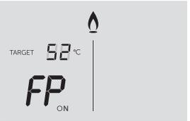
**Boiler is active for boiler frost protection:** operates if the ambient temperature is below 5°C until it reaches 19°C.
