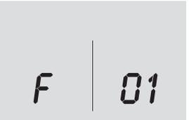
**Boiler has a fault for a specific error.** Display will show a number after the "F" to indicate which error is detected.
