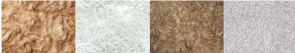
Cured glass mineral wool Blown glass mineral wool Rock mineral wool Wood wool
